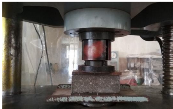
Fig. 6. Paving block under compression.
